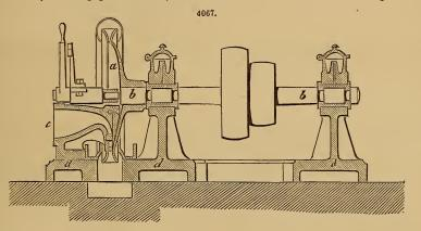
a horizontal shaft b b, which is provided with one or more pulleys. The water is brought through a pipe bolted upon the orifice c of the injector. The whole is erected upon a single bed-plate, which thus renders all the parts solid with each other. Fig. 4068 represents a large turbine which works directly and without gearing a horizontal
